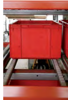
Roller strips and separator rails are individually adjustable
