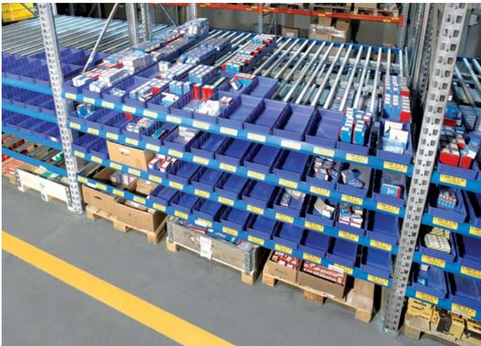
*The flow rack levels can be individually adapted to a very wide variety of container sizes*
