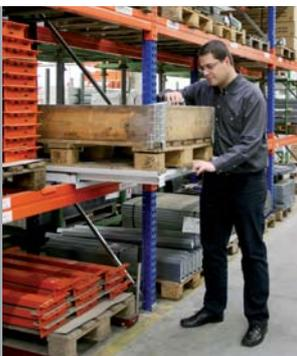
*Pallet drawers allow pallets to be pulled out effortlessly from the rack or on the floor*
