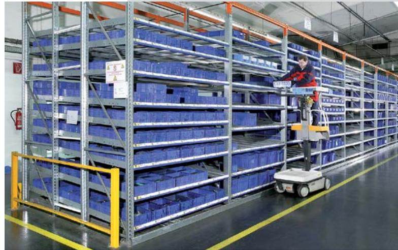
*META MULTILINE® L order picking flow rack with the FIFO principle (First In First Out)*
