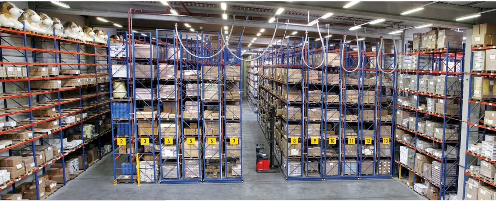
**With META mobile racks, you can either halve the warehouse surface area needed for the same storage capacity, or more than double your storage capacity!**
